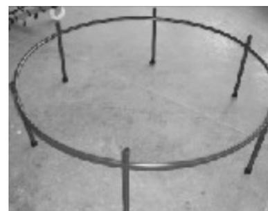
4. With the top rail frame connected into a circle, lay it flat on the floor (either side facing up, they are identical). Then insert the tapered end of each of the 6 leg tubes into the 6 leg sockets that are facing up, as shown.
